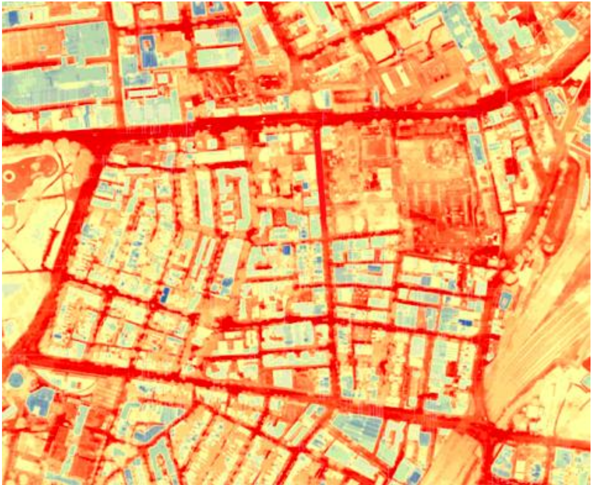
Figure 3 Infra-red image showing the increased heating effect of road surfaces compared to other structures in an urban setting
